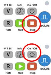
**Make sure the pump is powered off before replacing the battery.**
